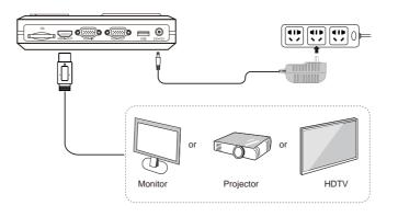
HDMI cable can be connected to monitor, projector, HDTV, and touch screen, etc.
